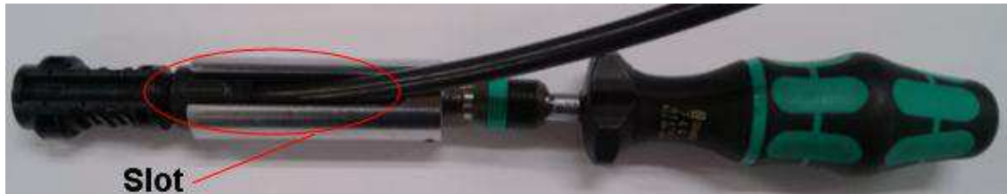
Figure 9 Tightening of the cable screw joint nut
